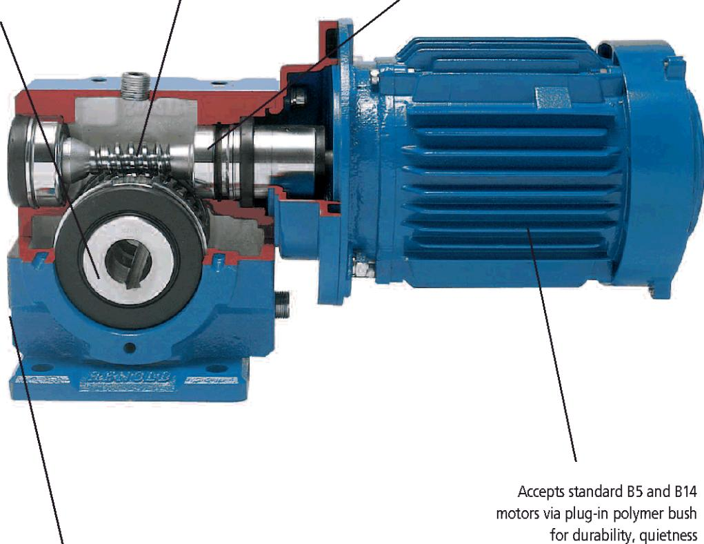
Machined surfaces on all sides of gear case, plus detachable feet and B5 output flange for wide range of mounting options.
